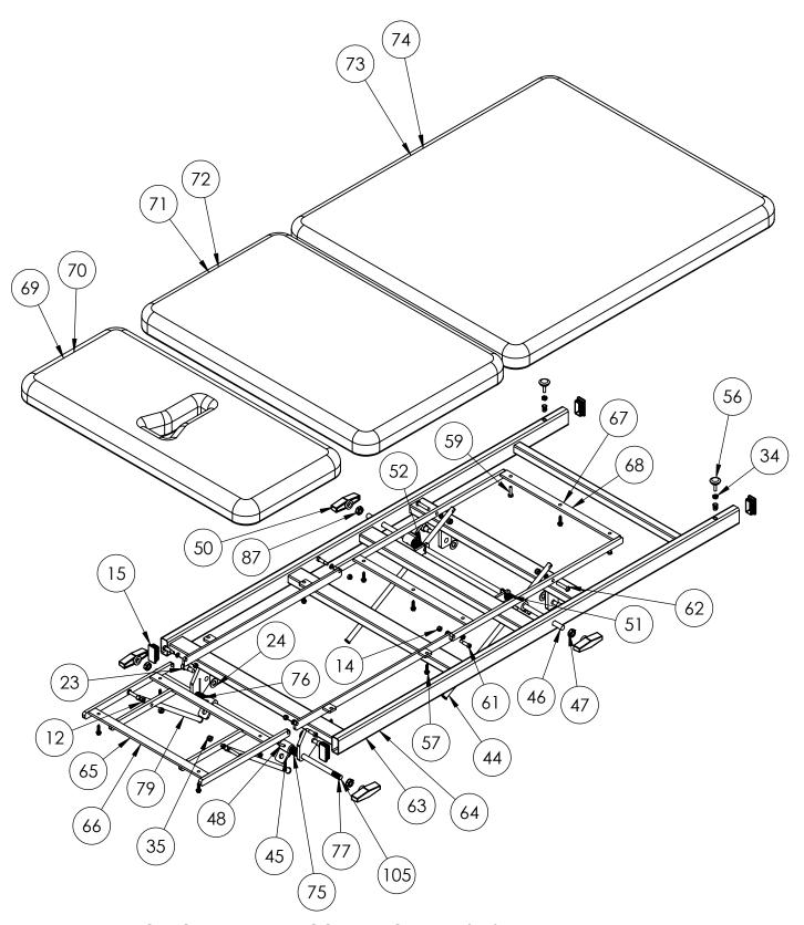
REFER TO MODEL NUMBER COLUMN ON PARTS LIST FOR ITEMS WITH TWO REFERENCE NUMBERS. EXAMPLE: ITEM NUMBER 73 IS USED ON AM-334. ITEM NUMBER 74 IS USED ON AM-340.
