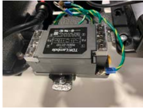
EMI Filter Secured Filter shown locked in place on the metal DIN rail.
