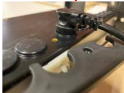
NOT Seated Gap between plug and control.
