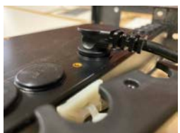
FULLY Seated No Gap between plug and control.
