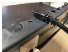
FULLY Seated Bracket setting OVER the cable plug and locks in place.
