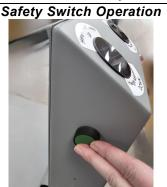
A safety switch is located on the side of the control tower, used to prevent unintended handrail movement.
