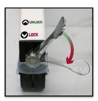
10) Unlock casters by lifting up on brake lever and roll EPD out of the way.
