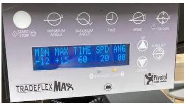
The Auto-Flexion User Interface displays the current Auto-Flexion parameters. The top line displays the parameter name, and the bottom line displays the current parameter.
